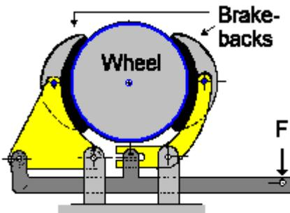
Figure 8:1: Mechanical brake assembly
