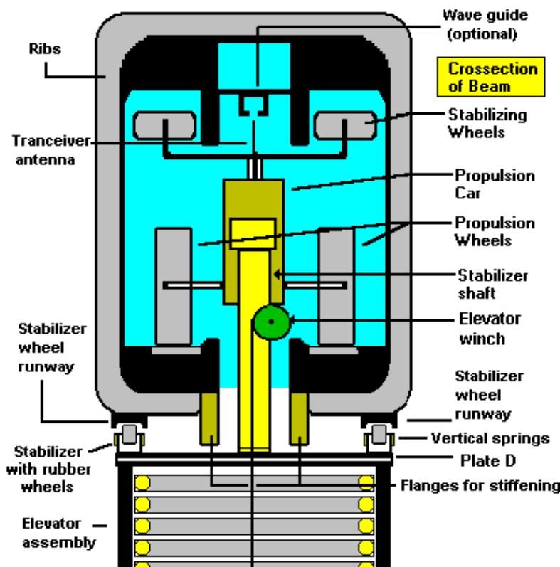
Figure 1:1: Cross-sectional view of beam and propulsion car
