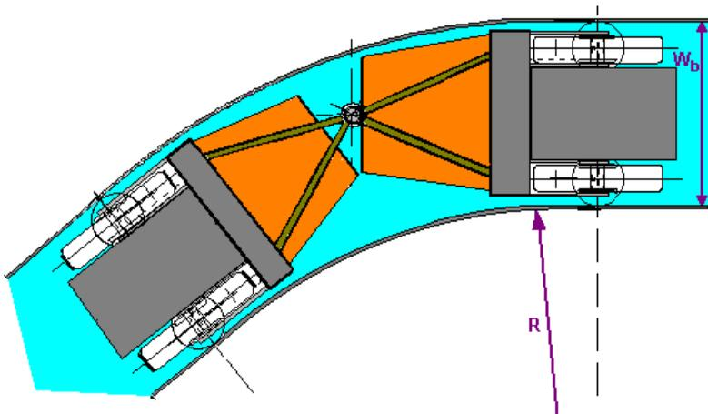
Figure 9:2: One pivot point, two platforms
