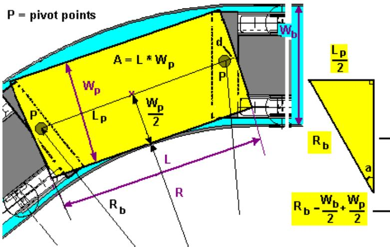
Figure 9:4: Trigonometry
