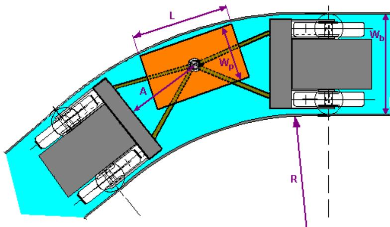
Figure 9:1: One pivot point, one platform
