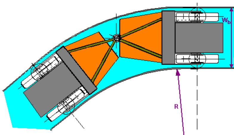
Figure 9:2: One pivot point, two platforms
