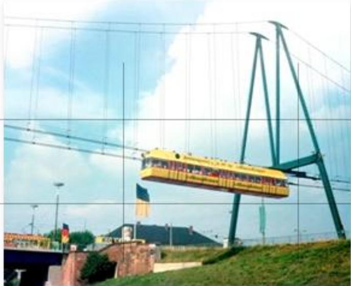
In place of a conventional monorail's massive, unsightly concrete support pillars, Aerobus utilizes slender steel pylons to elevate suspension cables, similar to those used in the Golden Gate Bridge.
