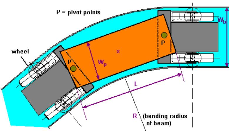
Figure 9:3: Two pivot points, one platform
