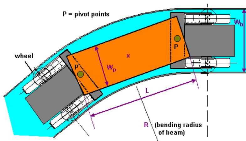
Figure 9:3: Two pivot points, one platform
