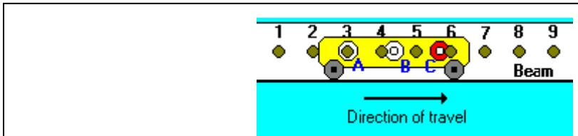
**Traction**, then, is only a limiting factor in the **first** case, i.e. when asynchronous motors for propelling the wheels are used. In this case, the slope of the beams are limited to  $5^\circ$ . If linear motors (LIMs) are used, traction is not a limiting factor, and the slope could be increased to  $10^\circ$ , possibly more.
