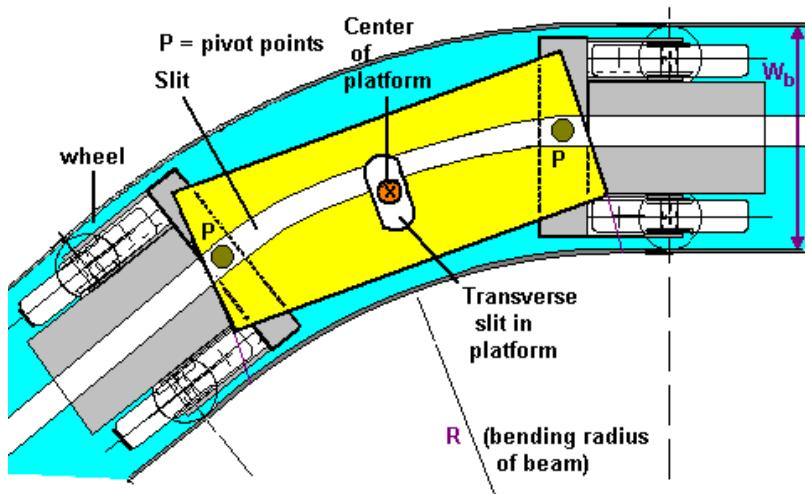
Figure 9:5: The slit in the Platform<sup>1</sup>
