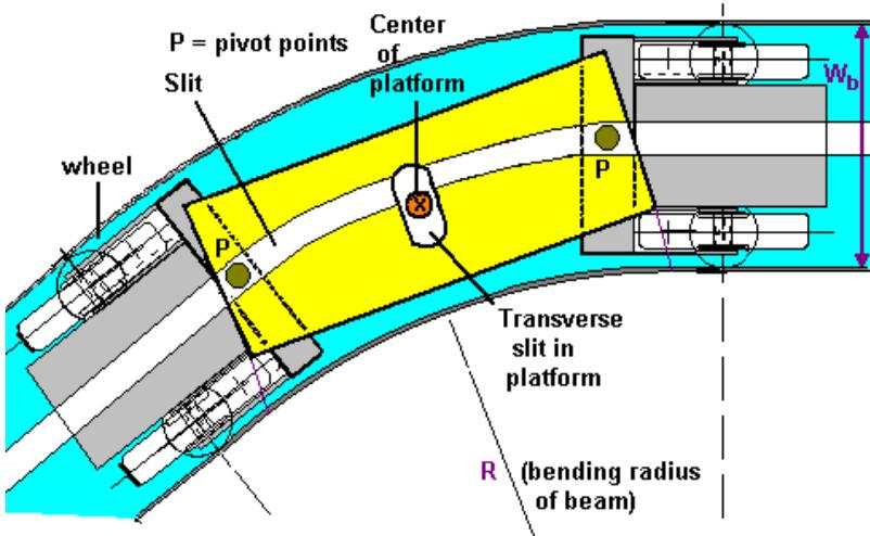
Figure 9:5: The slit in the Platform<sup>1</sup>
