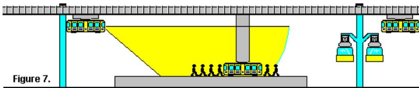
**Case A:** The car is brought to a halt from full speed, lowers the cabin, exchange passengers, lifts the cabin and accelerates to full speed.
