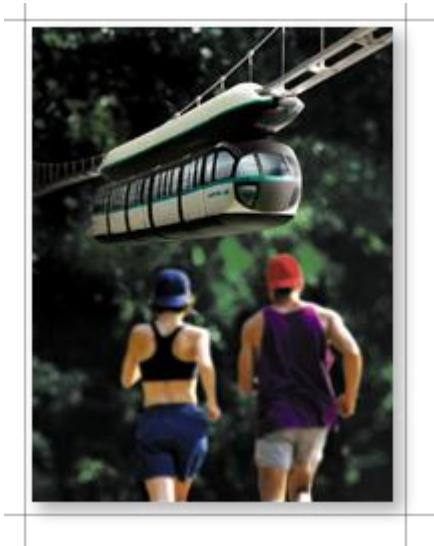
Each vehicle is self-propelled by safe, environmentally clean electric motors. Where needed, articulated vehicles may be used to permit tight turns in crowded or space-cramped settings.
