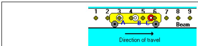
**Traction**, then, is only a limiting factor in the **first** case, i.e. when asynchronous motors for propelling the wheels are used. In this case, the slope of the beams are limited to 5°. If linear motors (LIMs) are used, traction is not a limiting factor, and the slope could be increased to 10°, possibly more.
