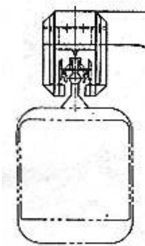
The Aerorail guideway rails are two #115 standard railroad rails with a 1m gauge. Wheels are 30" in diameter. As in other state-of-the-art transit systems, propulsion is by VVVF (Variable Voltage, Variable Frequency) 3-phase AC traction
