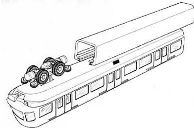
„The essence of the system was the conversion of the rubber-tired bogie developed for the Paris Metro into a bogie from which the coaches could be suspended to make an aerial railway. The bogie ran inside a hollow box girder on the lower
